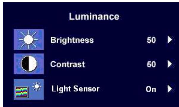
Press the ◀ or ▶ keys to adjust the degree of **Brightness**.
