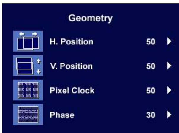
Press the ◀ or ▶ keys to adjust the display **Horizontal Position**.
